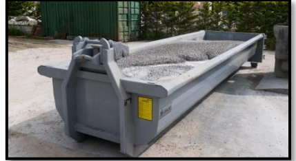
CEMBOX tipper with concrete waste
